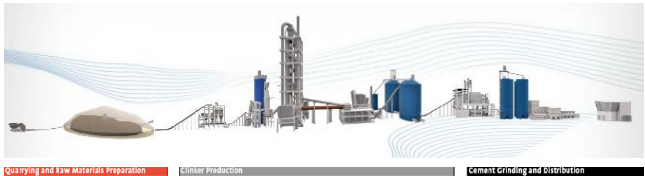
FIGURE 3 – FLOW SHEET OF DRY CEMENT MANUFACTURING PROCESS WITH STATE OF THE ART TECHNOLOGY
